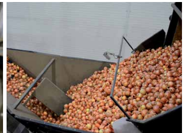
Product level sensor in a dosing bunker
