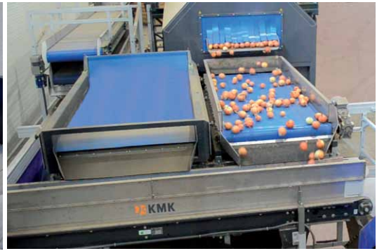
By-pass conveyor (moving left & right on a common frame with a machine)
