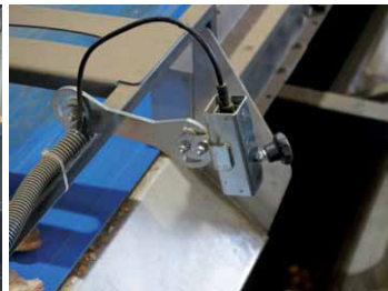
Product level sensor in an intake hopper of an elevator
